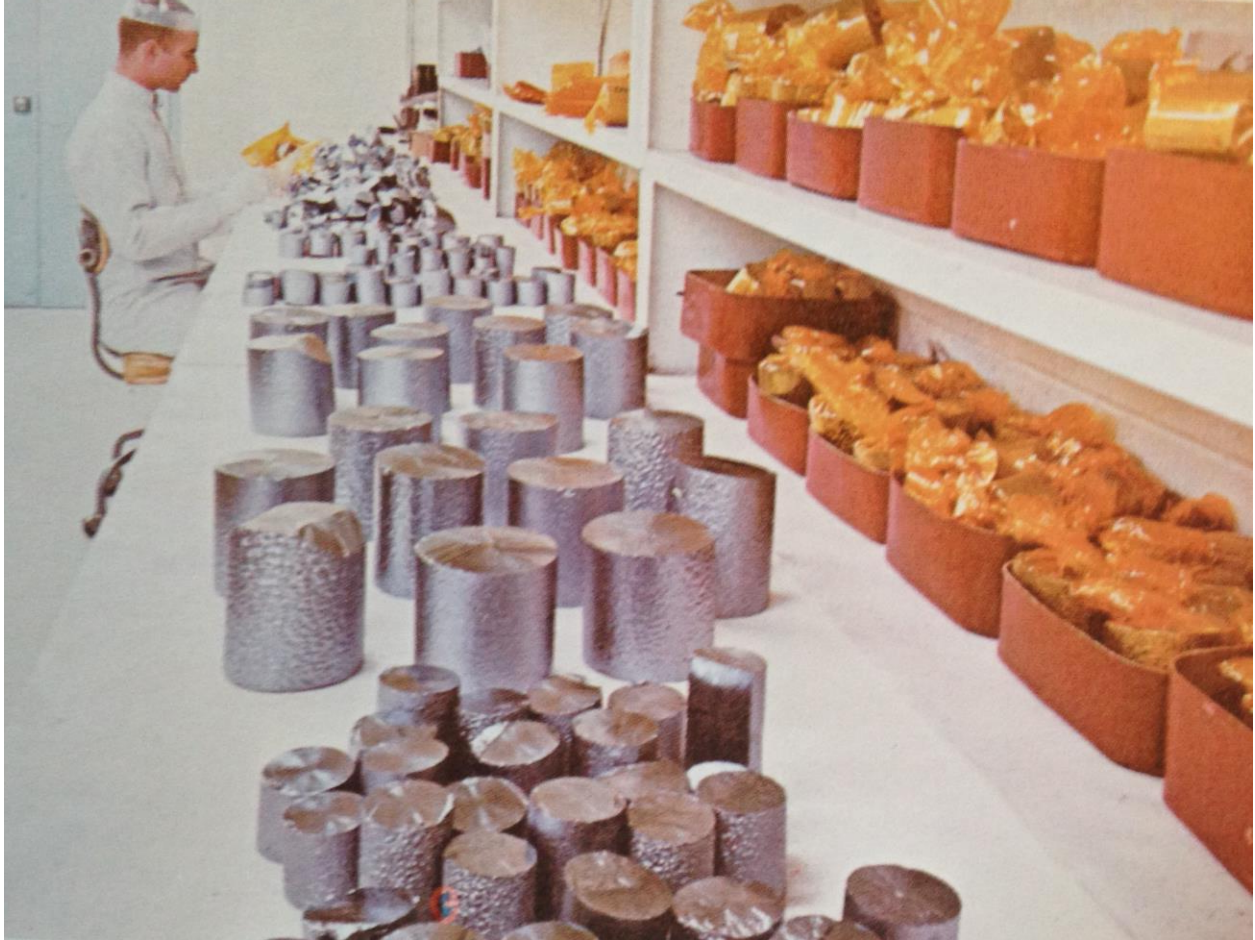
Figure 9. "TI's silicon reactors supplied the ultra-pure material for the crystal pullers. Silicon crystals were then sliced into thin wafers for use in transistor manufacturing." Pirtle, 70.
