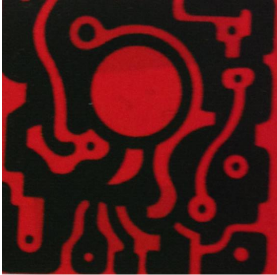
Figure 27. Sample of circuit board masking material attached to an advertisement for Rubylith by Ulano in Electronics 39 (June 13, 1966): 22. Ad copy included these phrases: "Making masks for Electronic Components," "Hand-cut masking firm for the graphic arts," and "the knife-cut light-safe masking film laminated to a stable polyester base." Image re-appeared in Prelinger, 108.
