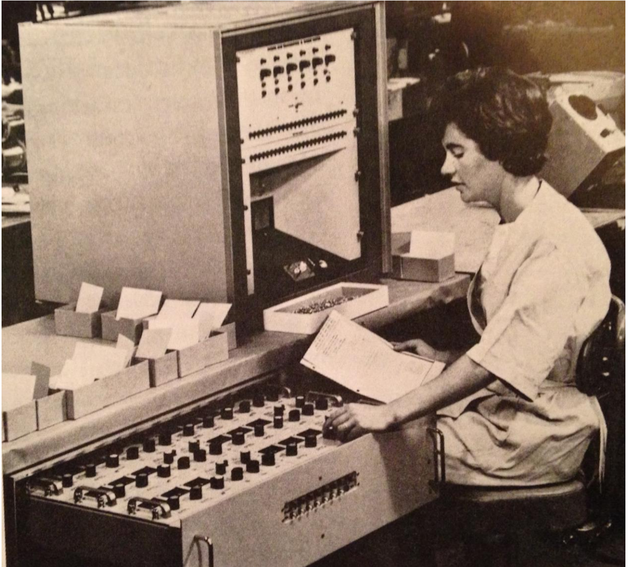
Figure 32. A Texas Instruments worker demonstrates equipment to test transistors and diodes. [ Electronics , 1964]. Image retrieved from Prelinger, 87.
