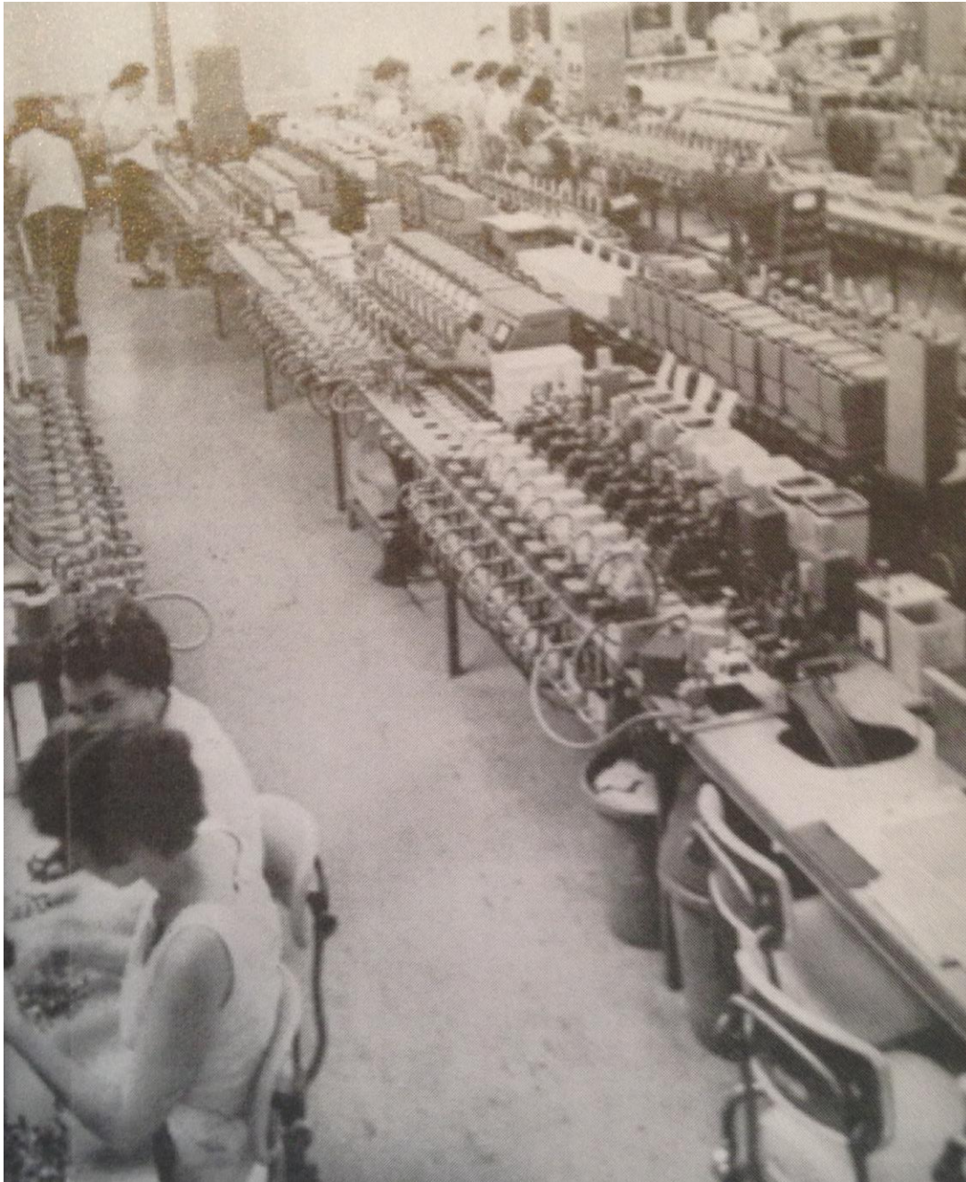
Figure 31. "Rows of Centralized Automatic Tester (CAT) machines testing transistors in the Semiconductor Building in 1960." Pirtle 78.
